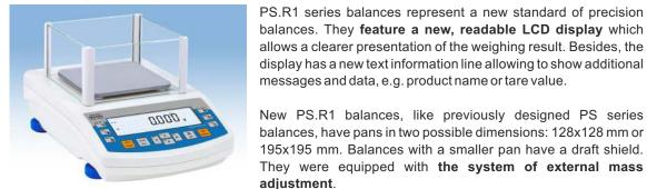
PS.R1 series balances represent a new standard of precision balances. They feature a new, readable LCD display which allows a clearer presentation of the weighing result. Besides, the display has a new text information line allowing to show additional messages and data, e.g. product name or tare value.
