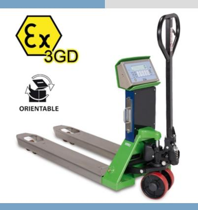
Pallet truck scales, with built-in electronic weighing, suitable for harsh working conditions and dangerous areas classified as hazardous (ZONE 2, 22) in accordance with Ex II 3GD IIC T6 T130°C X protection. The Atex certified four load cell weight detection guarantees the best accuracy in all work conditions. Available also CE-M APPROVED.
