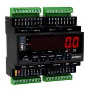
Digital weight transmitter designed specifically for use with digital weighbridge and silo weighing. It integrates functionalities for load cell addressing, quick replacement, equalisation and calibration. It provides diagnostics and weight readings for each connected load cell. Truck or silo weight can be sent to a PC via Fieldbus protocol, analog output or RS485. It can be used in legal for trade applications when combined with Rice Lake and Dini Argeo digital weighbridge load cells.
