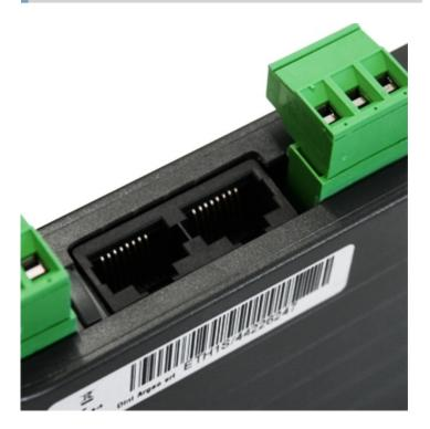
Thanks to Quick Connect system, the connections between DGT1S weight transmitter and the converter are simplified and speeden up.
