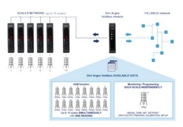
PROFIBUS FOR DIGITAL WEIGHING SCALES: CONFIGURATIONS (Please click on the image to enlarge)
