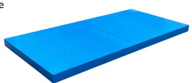
MWS follows simple strength by design principles and has manufactured the HCPM using 120 x 60mm box section with an 8mm deck plate. The ensures that the unit is strong enough to cope with loads up to 12,000kg while remaining just 160mm high.
