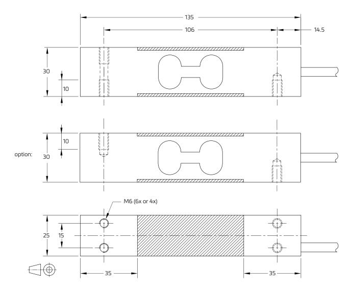
Mounting bolts M6 8.8; torque 10 Nm. Torque value assumes oiled threads.
