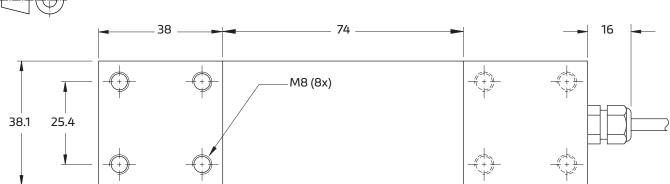
Mounting bolts M8 8.8; torque 25 Nm. Torque value assumes oiled threads.
