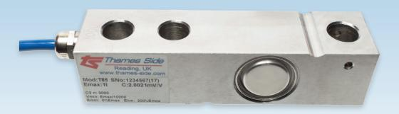
This stainless steel shear beam load cell is available with approval according to OIML R60 Class C3 (3000 divisions) and is calibrated in mV/V/ $\Omega$  by output current matching, which minimises corner correction time on multi-cell systems.
